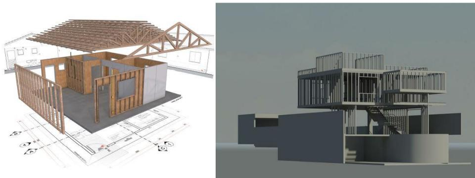
Figura 23 – Wood Framing e Steel Framing
